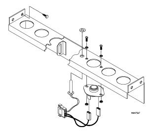
Disconnect sensor bracket harness connector.
